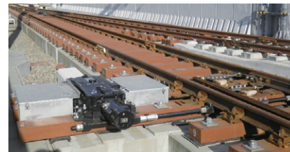
Railroad switch device (construction of overpass near Niigata Station)
